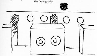
The diamiter of the mouth of one of the potts is  $5\frac{1}{4}$  Inches and 2 Inches &  $\frac{1}{2}$  from the mouth the diam is  $10\frac{1}{2}$ . The bottom 9 Ins. the Inside length  $17\frac{1}{2}$  Inches. The greatest Inside Diam. is 12 Inches The Inchnography "
